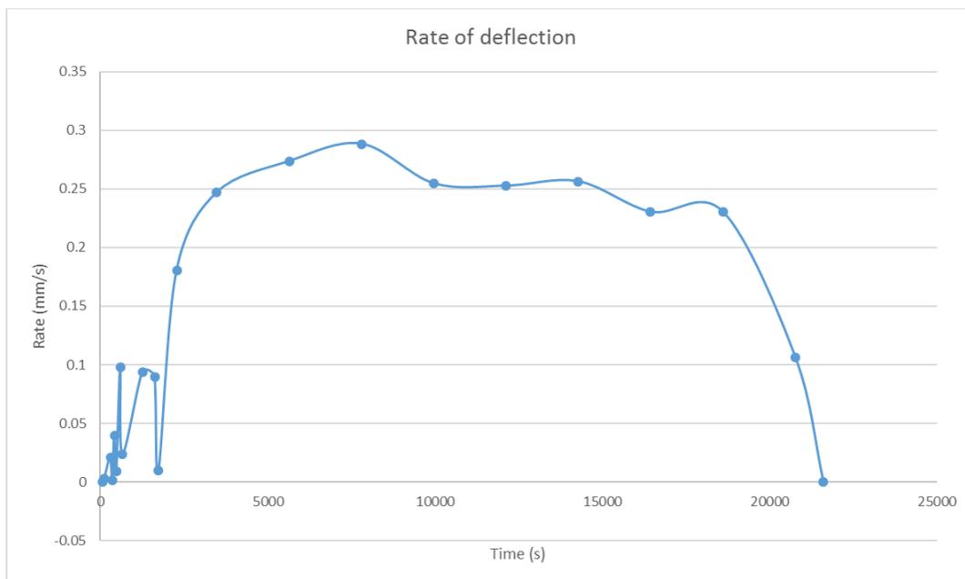
**Figure 71.** Rate of deflection (mm/s) vs Time (s) – Exposed side
