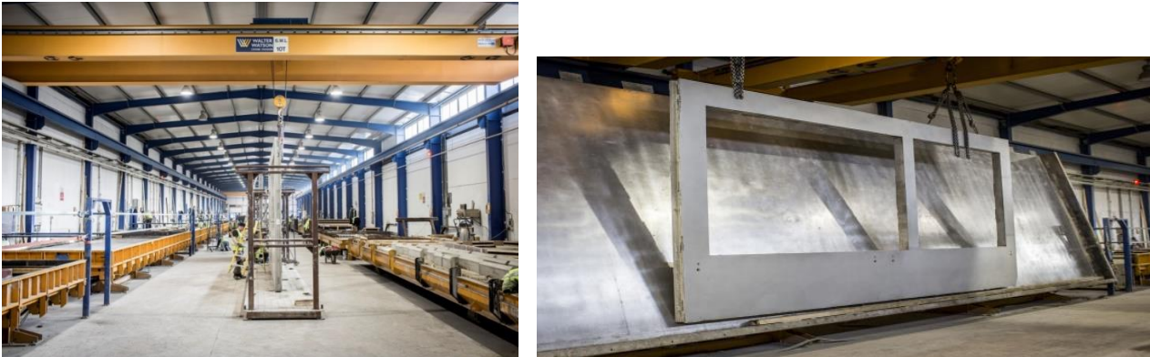
Figure 1: Creagh main factory in Toomebridge, Northern Ireland with tilting and vibrating heated tables.
