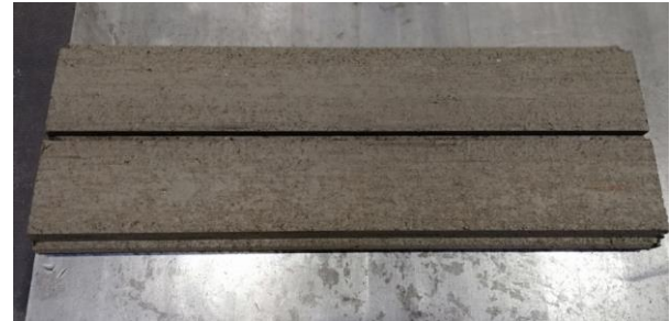
Figure 6 – Marmoroc® Baltic stones with 75% CDW replaced aggregate.
