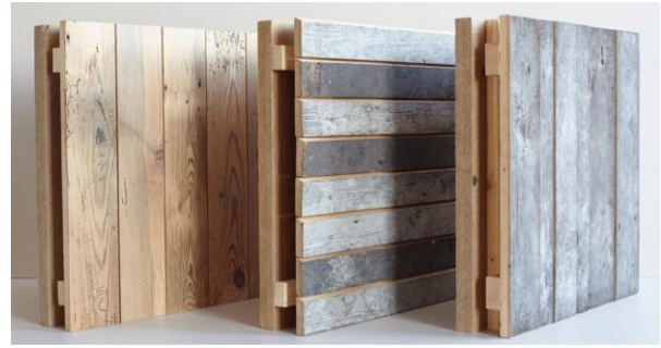
Figure 6: Examples of weatherboard made of CDW timber
