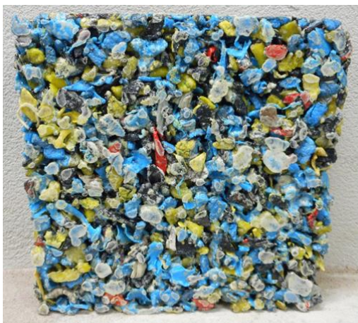
Figure 8: Insulation panel made of CDW rigid plastics
