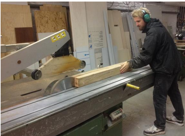
Figure 5: Lamella production for making timber beams
