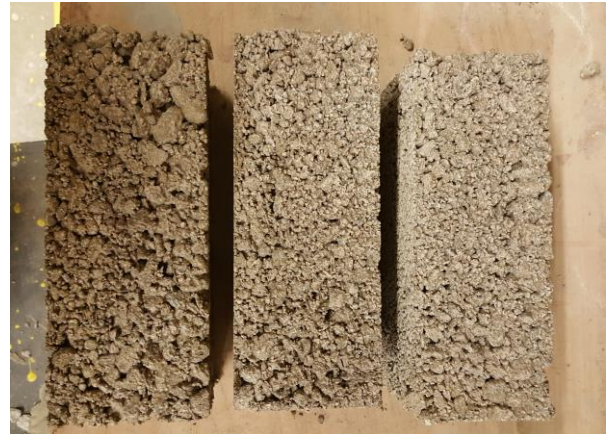
Figure 1: Building blocks made using a semi-dry mix
