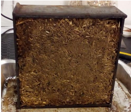
Figure 7: Insulation panel made of CDW wood fibres
