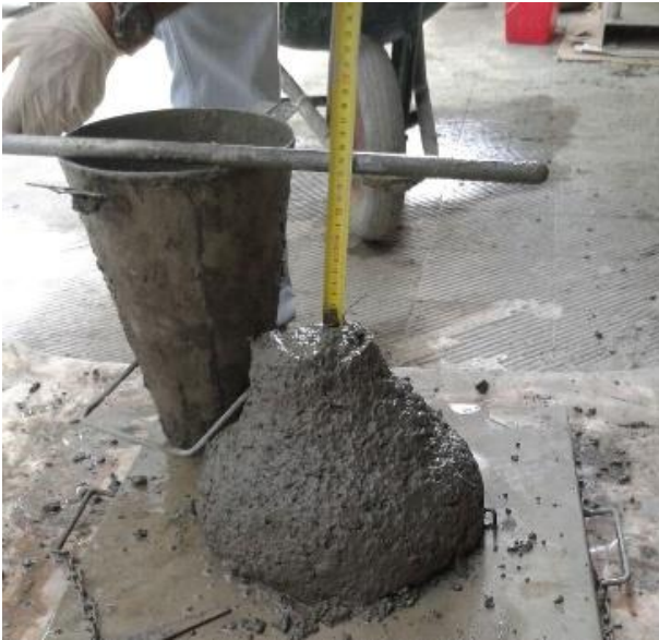
Figure 4 - Slump test on vibrated CDW/OPC concrete.
