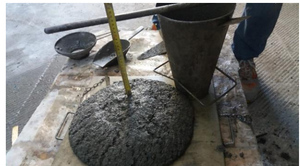
Figure 6 - Light-weight OPC concrete incorporating RP aggregates.
