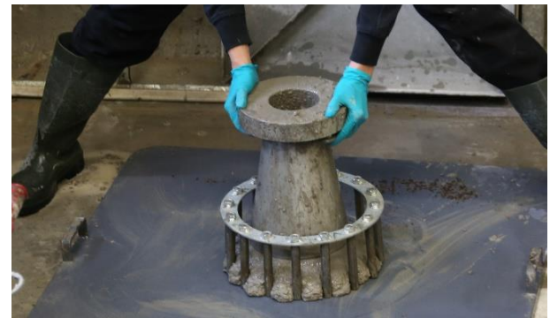
Figure 3 – J-ring test on self-compacting CDW/OPC concrete.
