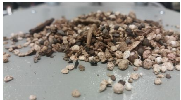
Figure 1 - RE 4 CDW used as aggregates for concretes development. Mineral fractions in three different sizes (0-2 mm, 2-8 mm and 8-16 mm), rigid plastic and wood and plastic fractions, respectively.
