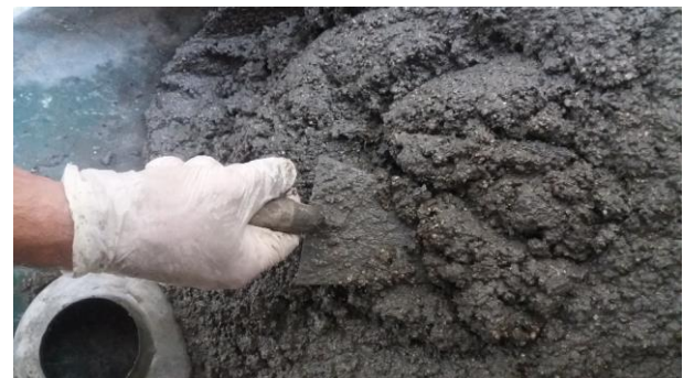
Figure 7 - Light-weight OPC concrete incorporating WP aggregates.
