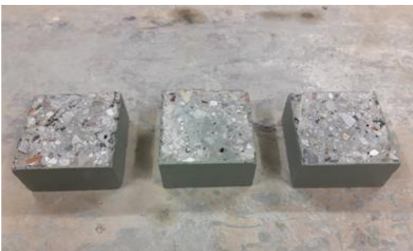
Figure 5 – Vibrated CDW/AAB concrete specimens.
