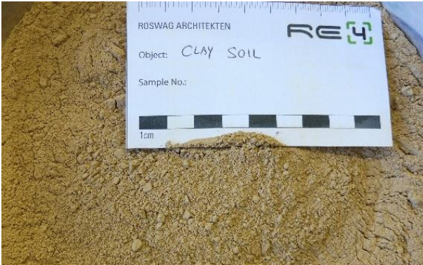
Figure 2 - Clayey soil used as binders for plasters/adhesives development.
