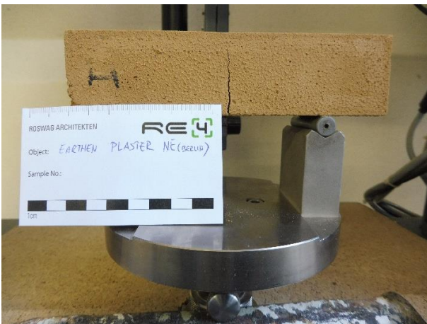
Figure 10 - Tensile strength test specimen.
