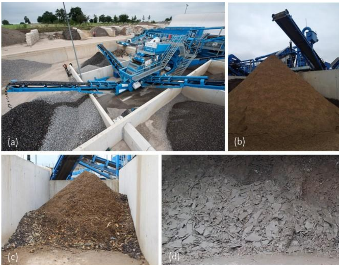
Figure 2.10: Typical output fractions resulting processing unsorted materials by CDE Global system: (a) C&D aggregates, (b) C&D sand (c) organic/lightweight mixed material, (d) silt/clay mixed materials.
