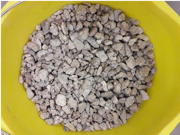
Fig. 18: Hand-picked mixed concrete/mineral aggregate (> 1.7 mm)
