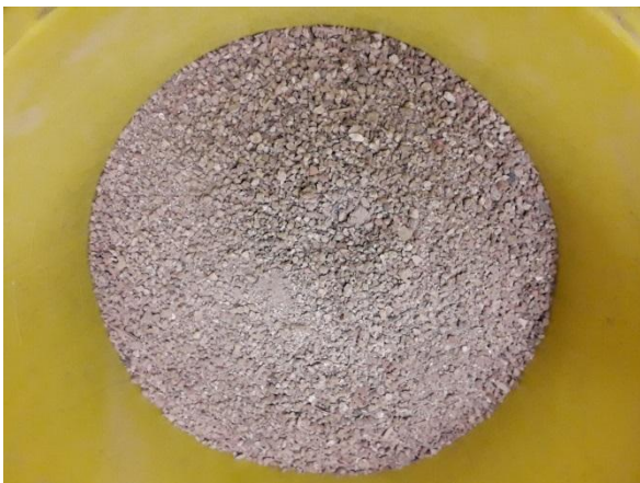
Fig. 22: Medium/coarse sand (0.6-4 mm) fraction
