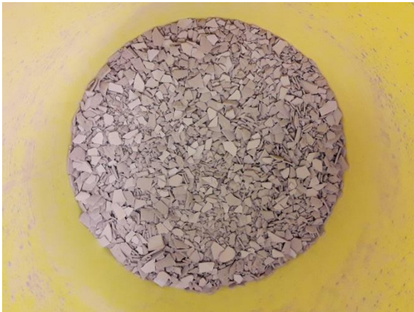
Fig. 25: Silt/clay (< 0.075 mm) sample
