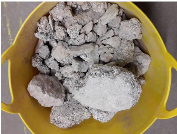
Fig. 26: Mixed concrete/mineral aggregate (> 20 mm) fraction
