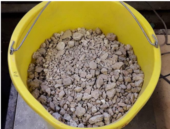
Fig. 4: Hand-picked mixed concrete/mineral aggregate (> 1.7 mm)
