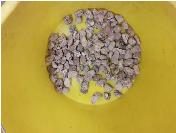
Fig. 19: Mixed concrete/mineral aggregate (16-20 mm) fraction
