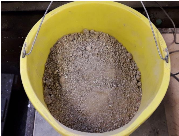
Fig. 8: Medium/coarse sand (0.6-4 mm) fraction
