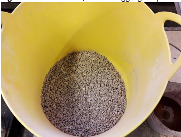
Fig. 7: Mixed concrete/mineral aggregate (4-8 mm) fraction
