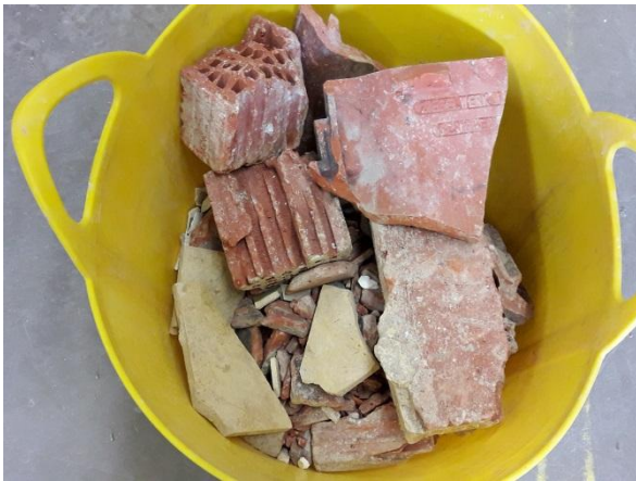
Fig. 28: Ceramics (bricks and tiles > 1.7 mm) fraction
