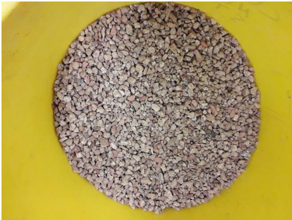
Fig. 21: Mixed concrete/mineral aggregate (4-8 mm) fraction
