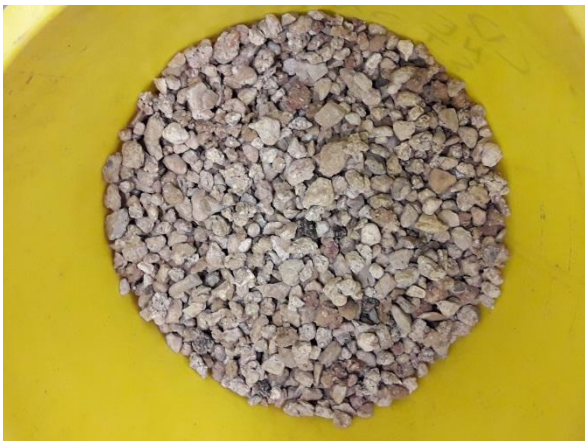
Fig. 20: Mixed concrete/mineral aggregate (8-16 mm) fraction
