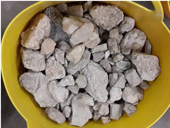
Fig. 12: Mixed concrete/mineral aggregate (> 20 mm) fraction
