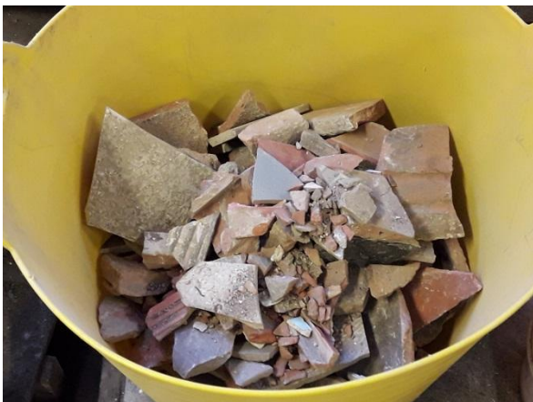
Fig. 14: Ceramics (bricks and tiles > 1.7 mm) fraction
