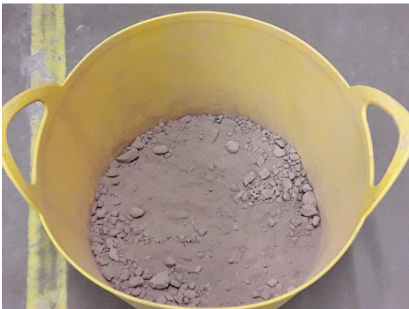
Fig. 9: Fine CDW material (< 0.6 mm)
