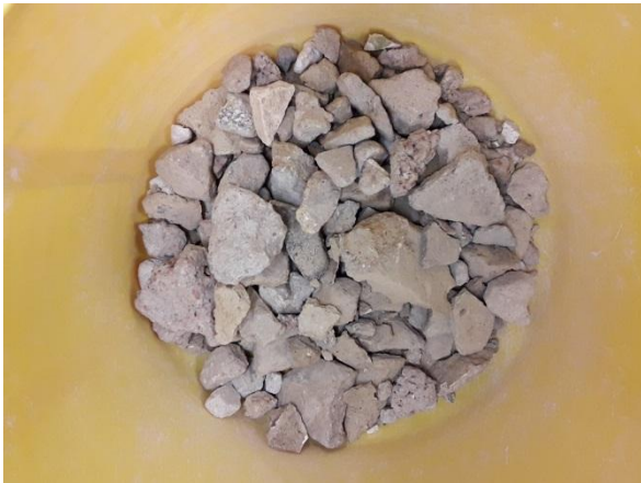
Fig. 27: Mixed mortar/plaster (> 1.7 mm) fraction
