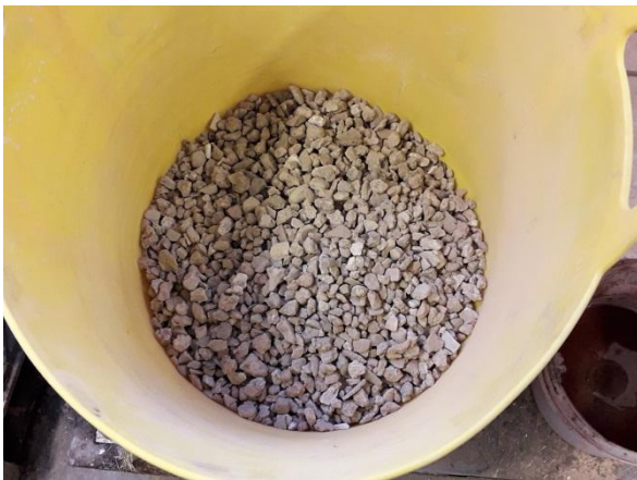
Fig. 6: Mixed concrete/mineral aggregate (8-16 mm) fraction
