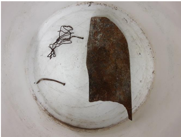
Fig. 31: Steel (nails, wire, pipe fragments > 1.7 mm) fraction
