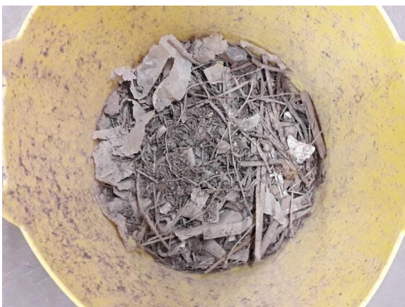
Fig. 17: Lightweight (mixed wood/plastics > 1.7 mm) fraction
