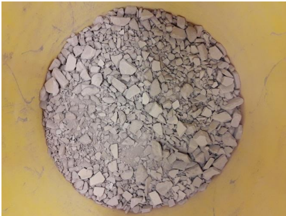
Fig. 23: Fine CDW material (< 0.6 mm)
