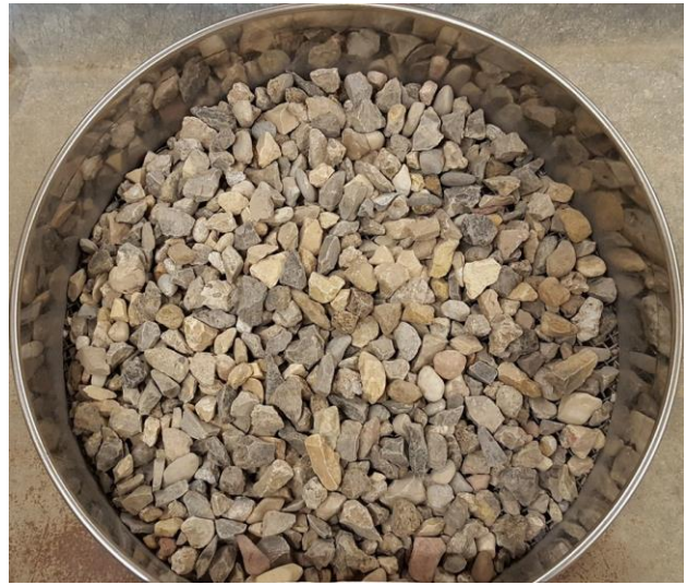
Figure 57 State of N.E.I.S. mineral fractions after 10 freeze-thaw cycles.
