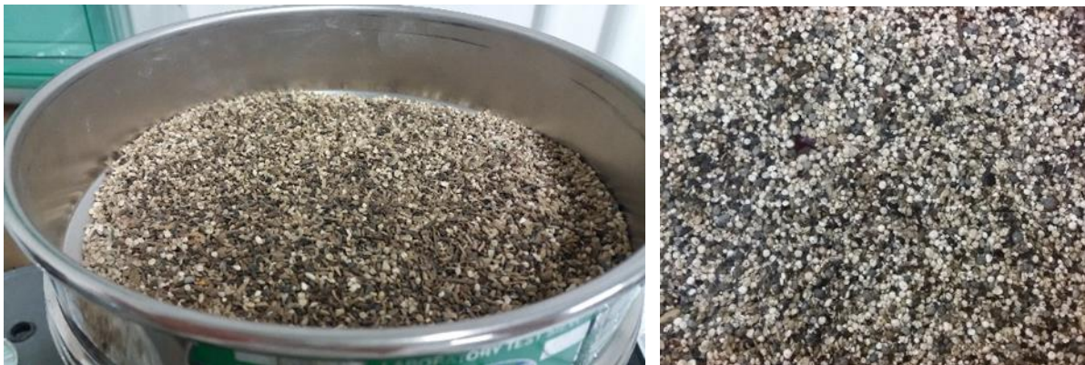
Figure 22 Wood and Plastic fractions rejected from CDW processing plants and relevant magnification (on the right) showing polystyrene particles and cortex pieces.
