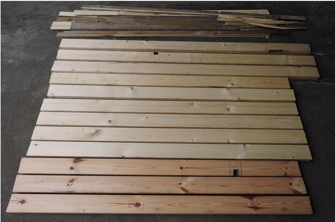
Cut and planed lamellas ready for strength grading. The marked areas need to be cut out, due to impurities.
