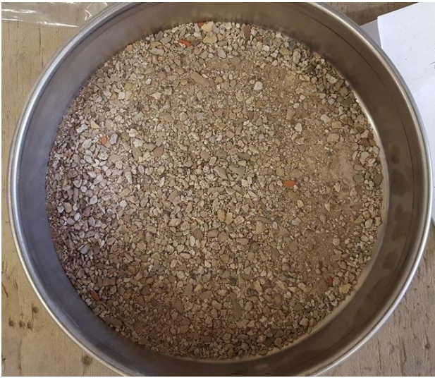
Figure 60 N.E.S. fine particles (< 4 mm) collected after the end of 10 freeze-thaw cycles.
