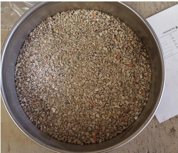
Figure 62 S.E.S. fine particles (< 4 mm) collected after the end of 10 freeze-thaw cycles.
