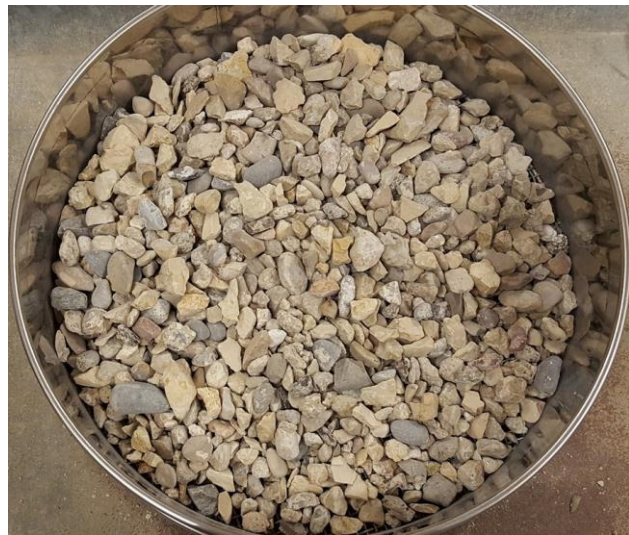
Figure 59 State of S.E.I.S. mineral fractions after 10 freeze-thaw cycles.
