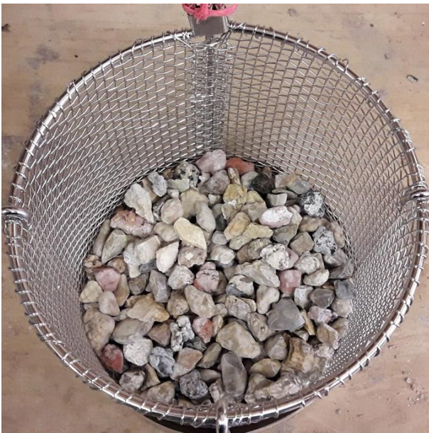
Figure 13 Coarse S.E.S. aggregate sample placed inside mesh baskets for performing the MgSO_4 test.
