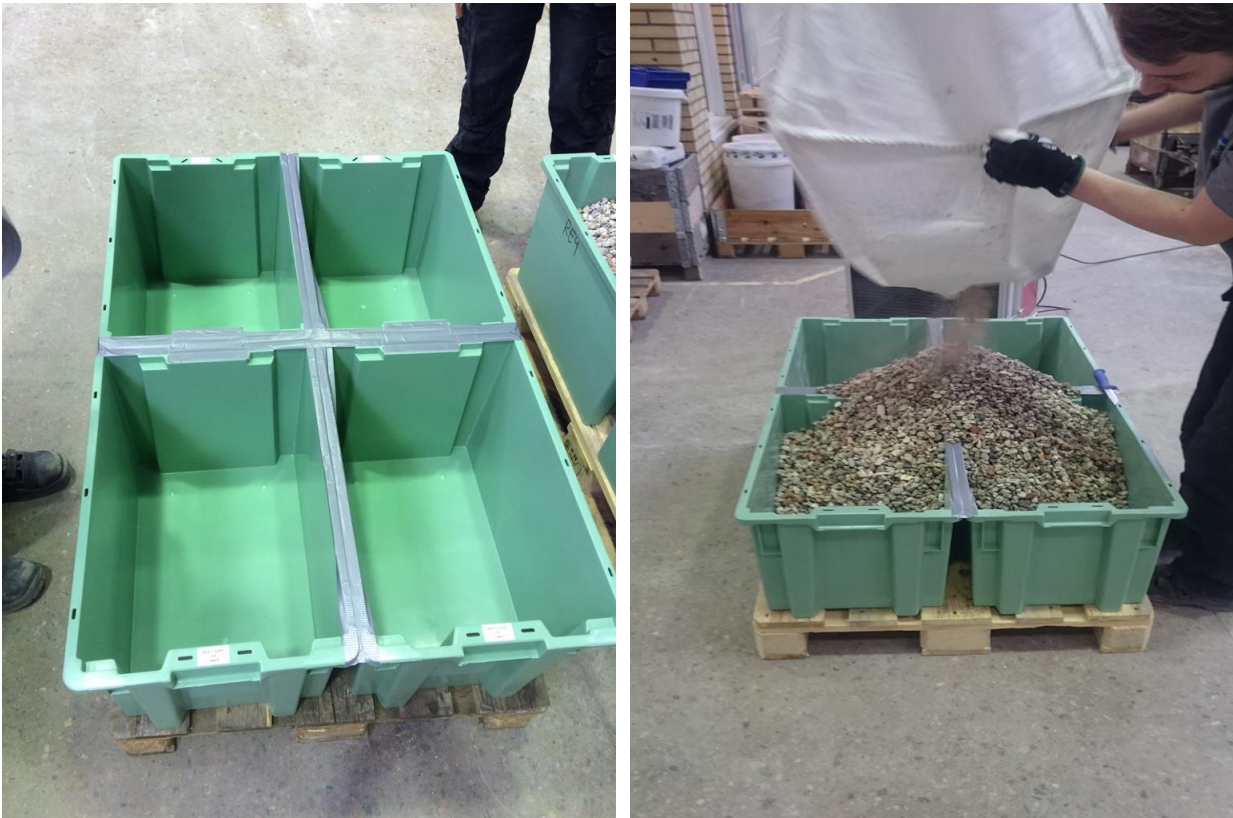
Figure 1 Reduction of large amounts of 8/16 S.E.S. mineral fraction, using four rigid plastic containers on a pallet.
