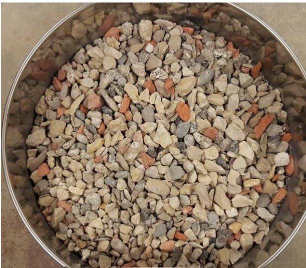
Figure 58 State of S.E.S. mineral fractions after 10 freeze-thaw cycles.
