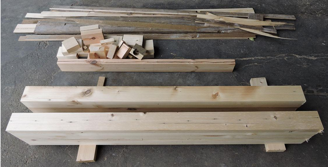
Reprocessed lamellas, one lamella has been rejected due to cracks, some impurities have been cut out.
