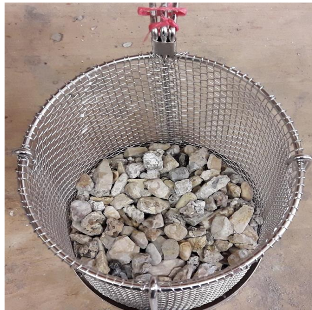
Figure 14 Coarse S.E.I.S. aggregate sample placed inside mesh baskets for performing the MgSO_4 test.
