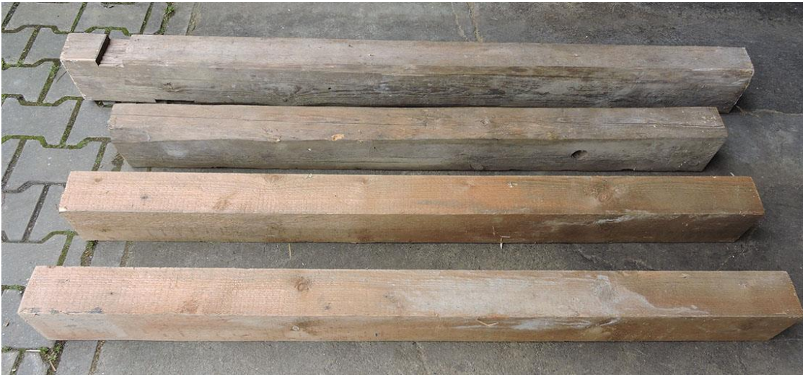
Timber beams ready for reprocessing, cleaned of nails and cut in half for logistic reasons. Amount 0,08m 3 salvaged timber.
