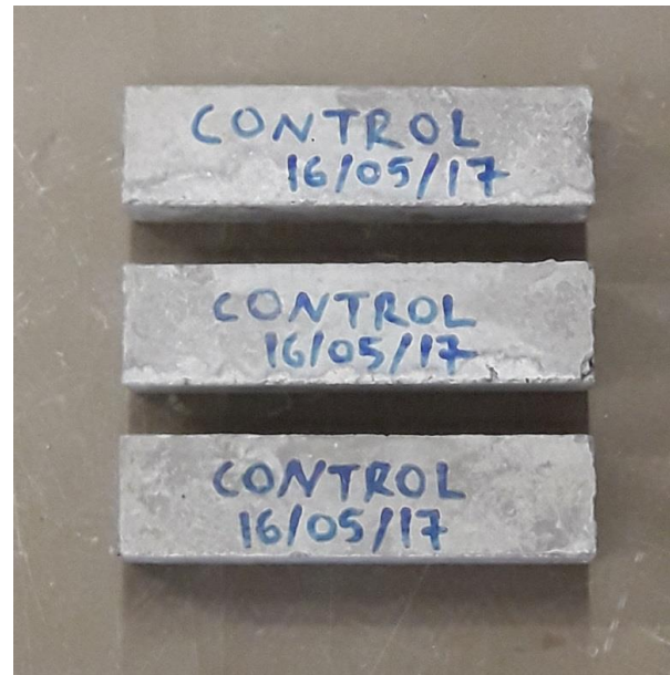
Figure 16 Concrete prisms for drying shrinkage testing (control specimens).
