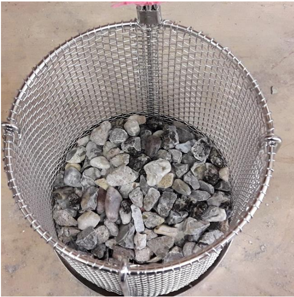
Figure 11 Coarse N.E.S. aggregate sample placed inside mesh baskets for performing the MgSO_4 test.
