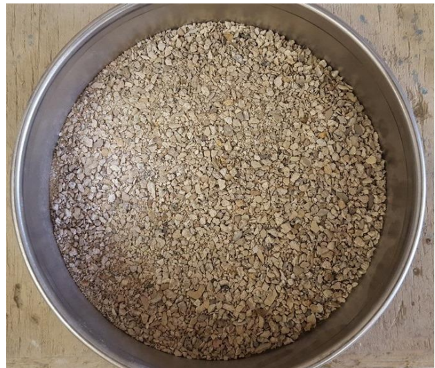
Figure 63 S.E.I.S. fine particles (< 4 mm) collected after the end of 10 freeze-thaw cycles.
