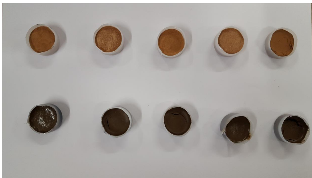
Figure 81 Visual observation of the uncalcined (bottom) and calcined (top) fine material.
