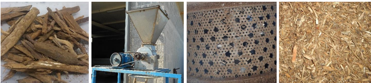
Figure 25 Wood fractions from S-EU source as received, grinder, 20 mm circular mesh sieve and wood after grinding process (size <20 mm).
