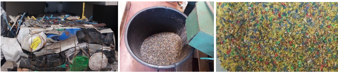
Figure 24 Rigid Plastic fractions from N-EU source as received, grinding process and resulting material (fine fraction).
