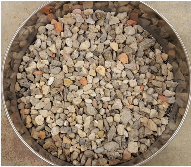
Figure 56 State of N.E.S mineral fractions after 10 freeze-thaw cycles.
