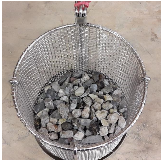
Figure 12 Coarse N.E.I.S. aggregate sample placed inside mesh baskets for performing the MgSO_4 test.
