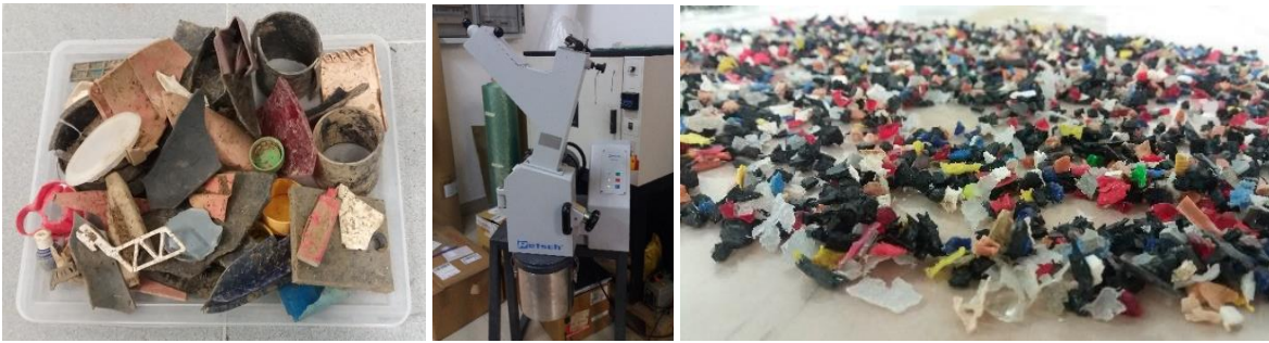
Figure 23 Rigid Plastic fractions from S-EU source as received, grinder and after the grinding process (coarse fraction).
