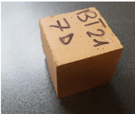
Figure 3 – Cured 50 mm Mortar Cube Made with Brick and Tile Waste
