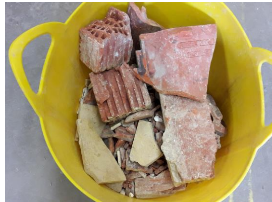
Figure 1 - Manually Sorted Brick and Tile Waste
