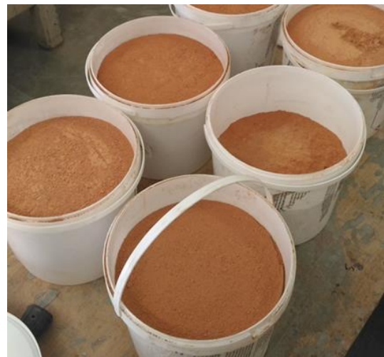
Figure 2 - Ground Brick and Tile Waste
