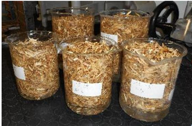
Figure 30: Absorption characterisation of 0-4 mm mixed sourced N-EU material
