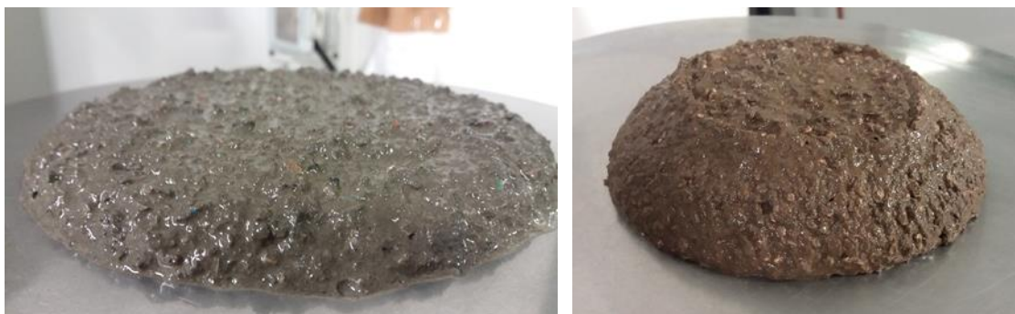
Figure 26: Mortars based on RE 4 lightweight fractions, Rigid Plastic and Wood and Plastic from N-EU.
