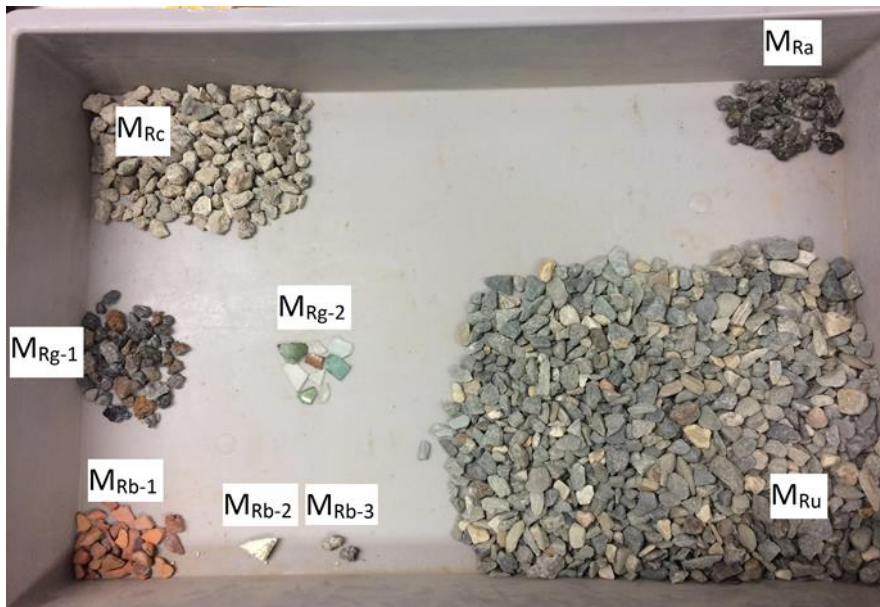
Figure 18: Constituent classification of 8/16 mm size fraction - S-EU Batch 2
